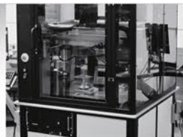
Large-size & Multiple Camera AOI for TFTs/LCDs
