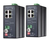
The EIP2-EXTEND-M & EIP2-EXTEND-R are Industrial Long Reach Power over Ethernet Extenders to utilize existing copper cabling
